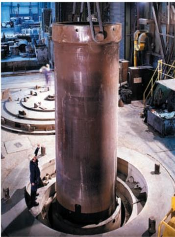
After the vertical spincasting process (VSP) became the standard at GP for indefinite chill and high-chromium qualities, it was also increasingly used for composite casting of working and back-up rolls.
