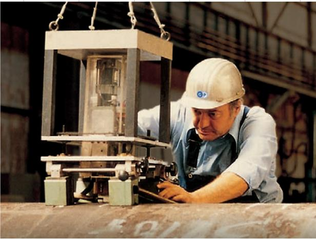
Electro-chemical measuring point preparation or 'ECM' has been used to determine tension, hardness, and residual austenites at GP since 1978. This inspection and testing method has made a decisive contribution to improved quality.
