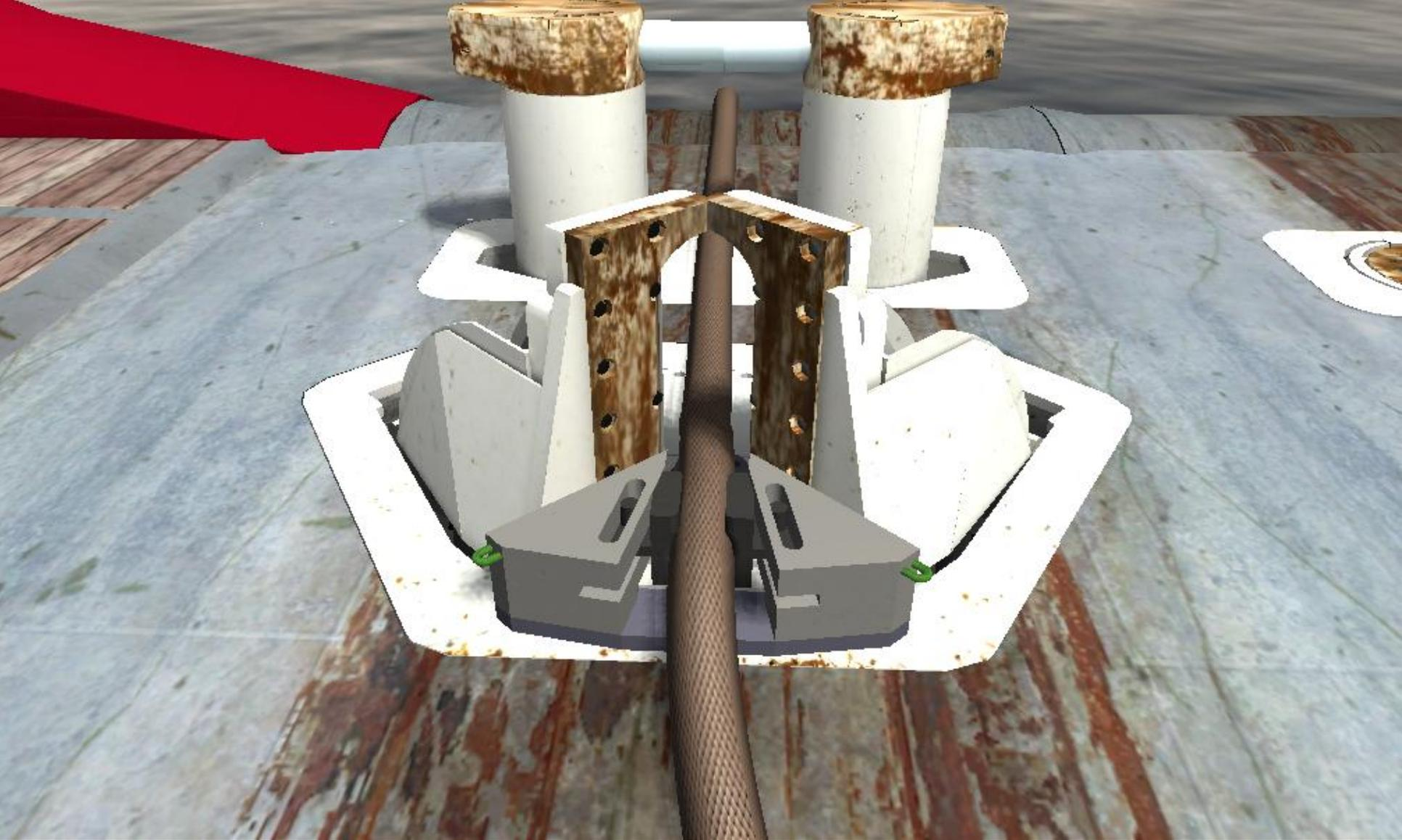
**Triples RFS** (Rope Friction Stopper)
